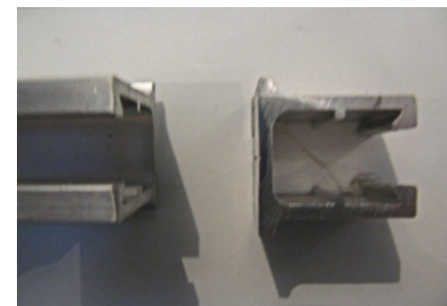
1" x 1" x 12" long medium channel (SIGNFIX) extrusion welded to backside of panel (Painted to match sign panel w/ a satin finish)
