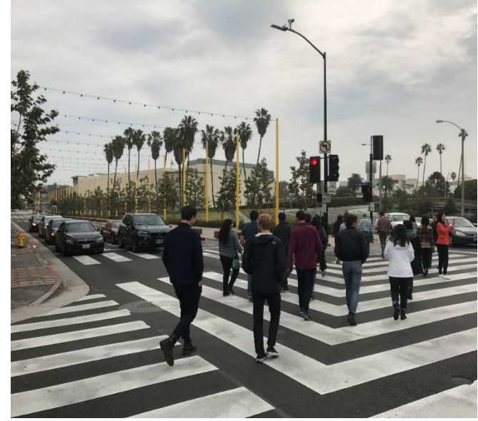
All-Direction Pedestrian Scramble Crossing Treatment, Santa Monica
