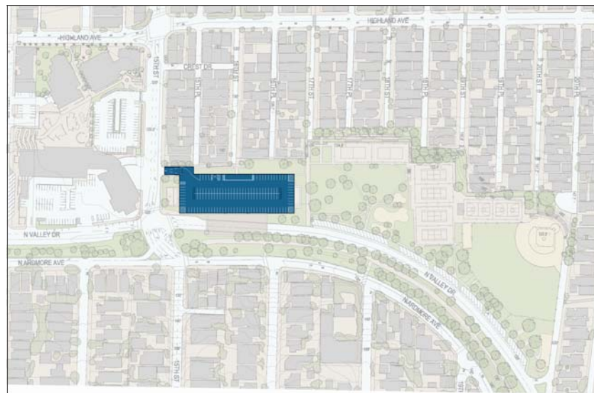
Live Oak Park Below Grade Parking in the Illustrative Plan. One hundred and thirty spaces are provided in a single level beneath the library and community center. The structure is accessed via a ramp at 15th street.
