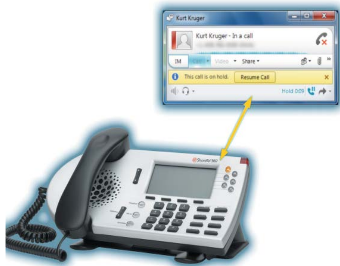
Example of a phone put on hold with the desktop application showing the same action.
