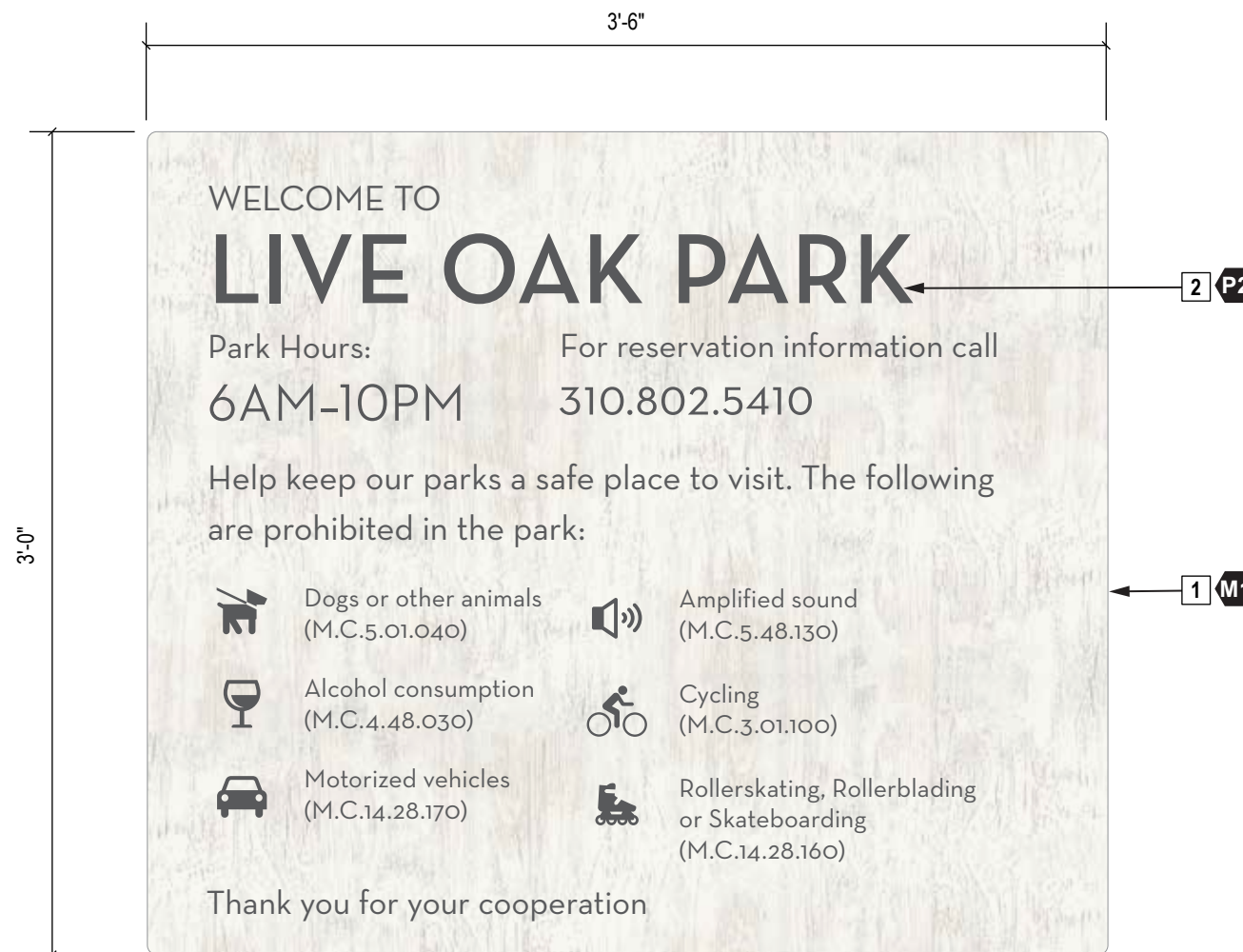
2 SIGN DETAIL - FENCE MOUNTED scale: 3/4" = 1' -0"
