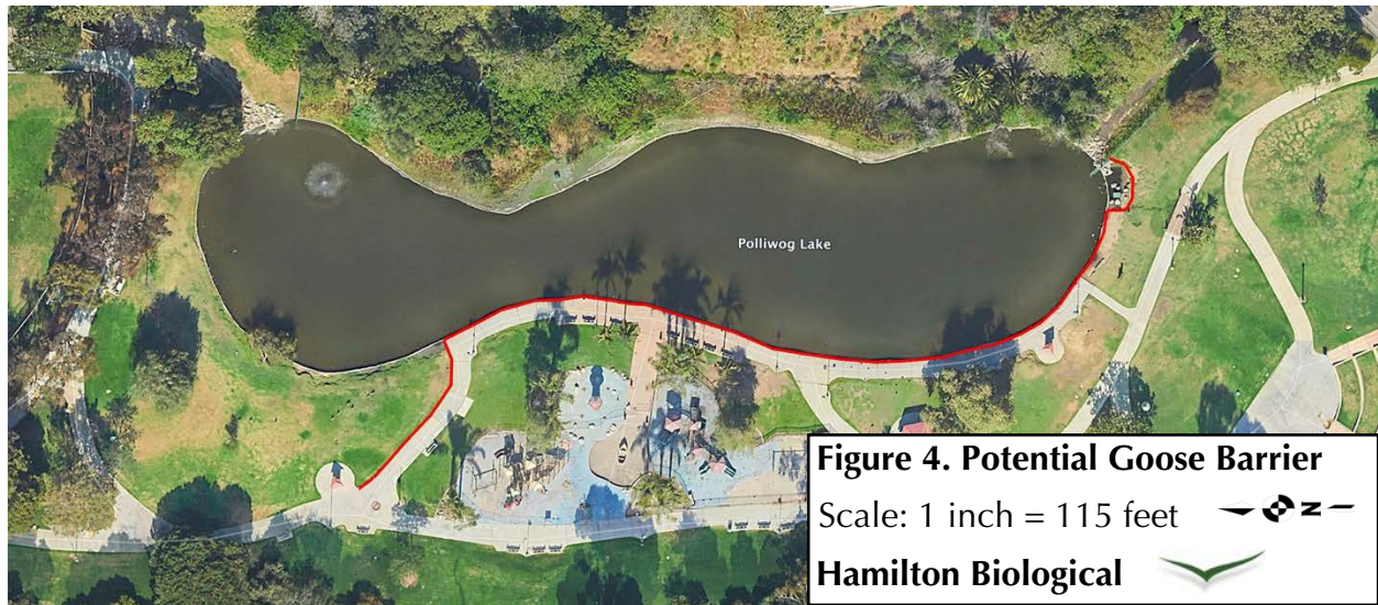
Figure 4. The red line represents, schematically, 570 linear feet of a low barrier, 36–48 inches tall, that could be established along the western and southern edges of Polliwog Lake, to discourage Canada Geese from congregating along the concrete walkway near the play area, or foraging in the amphitheater area. The geese and other waterfowl would still have unfettered access to areas of turf in the northern part of the park, which is used less heavily by members of the public. Source: Google Earth Pro.
