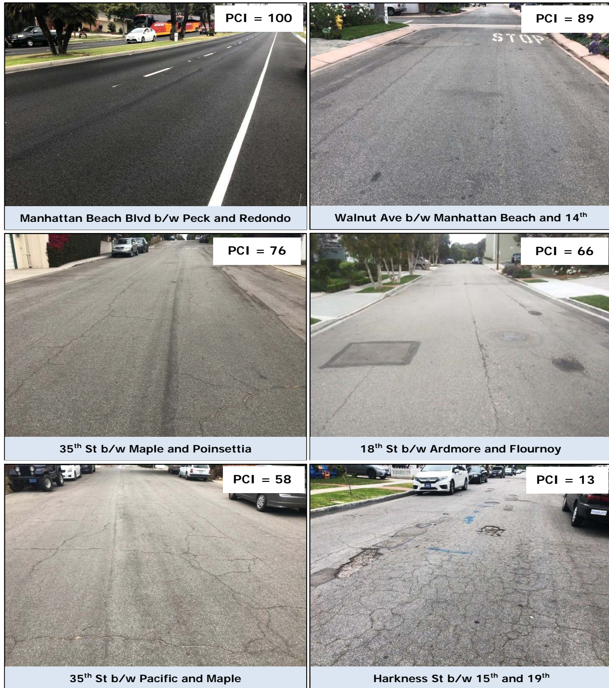
Figure 4: Examples of AC Streets with Different PCIs
