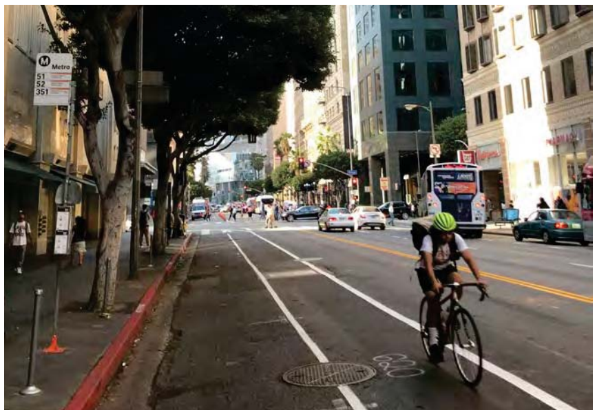
A mid-block bus stop where stopping buses must obstruct the bike lane while picking up or dropping off passengers
