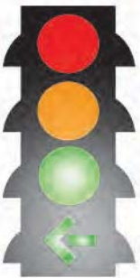
Protected-permissive left-turn signal
