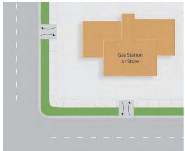
Reconstructed corner with fewer, narrower driveways (Credit: Michele Weisbart)
