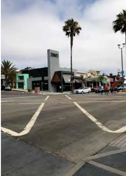
Pedestrian scramble at the intersection of Pier Avenue and Hermosa Avenue in Hermosa Beach.
