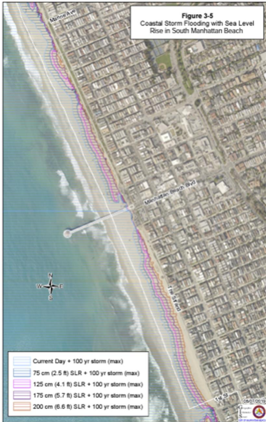
Figure 20: Coastal Storm Flooding with Sea Level Rise, S. Manhattan Beach
