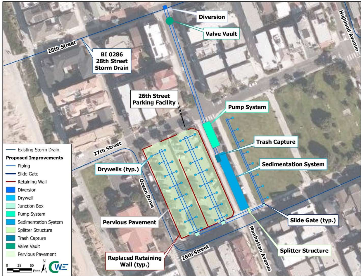
Figure 2-3 Stormwater Infiltration Concept
